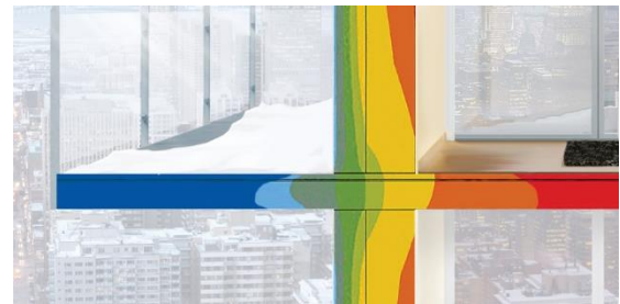
Figure 3 – Thermal Bridging at a Slab Balcony
