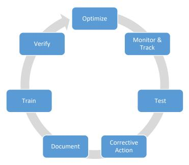
Ongoing commissioning is a **cyclical process** intended to be implemented over the life of a building. It allows building operations staff to gain insights on performance and allow for **predictive analysis and proactive action** rather than reactive maintenance and repair [4, 5].
